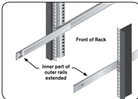
**CAUTION:** Failure to engage the ball-bearing assembly with the plastic guide (as shown below) can cause damage to your rail.
