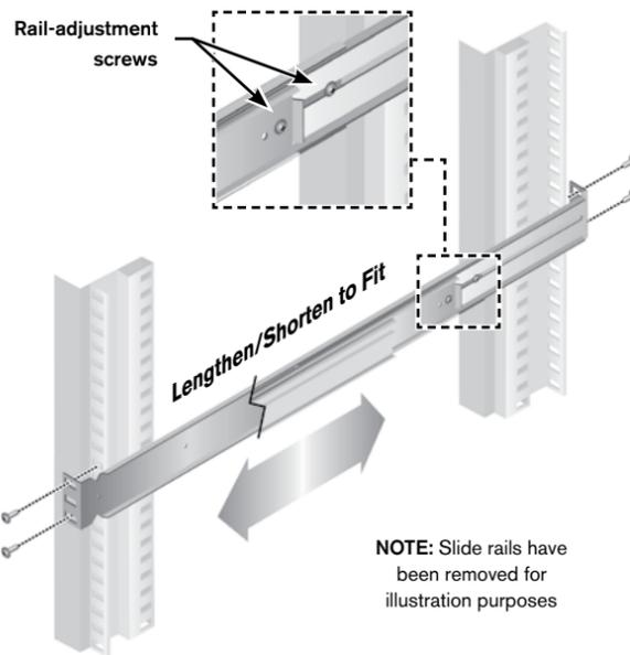
Loosely attach the back of the slide-rail brackets to the rack cabinet, using four screws. Ensure that the slide-rail brackets extend outside of the rack-cabinet mounting flanges. Tighten the two rail-adjustment screws on each of the outer rails.
