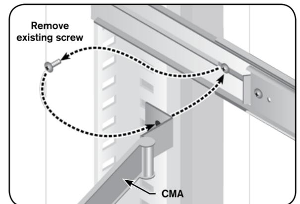
of the cable retractor arm. Align the cable-management arm (CMA) to the outer slide-rail bracket, and use the removed screw to attach the CMA.
