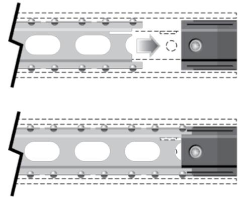
Carefully slide the LCD Tray into the ball-bearing assemblies in the rails.
