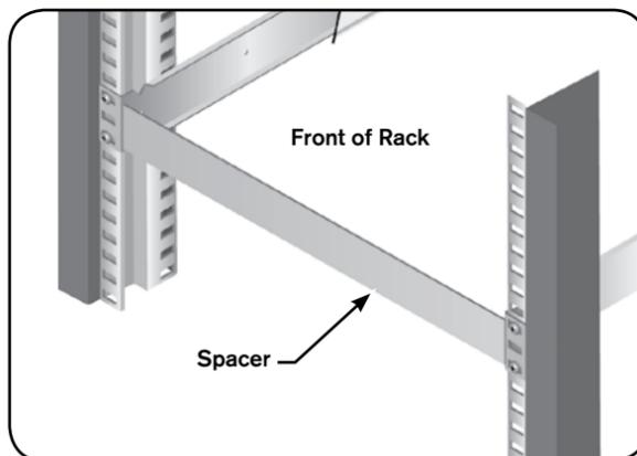
Brackets must fit snugly against the ends of the spacer to establish proper gap. Tighten the front four screws and remove the spacer.
