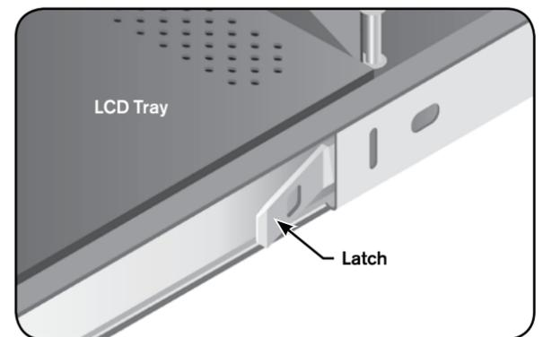
as the ball-bearing assemblies align between the inner and outer rails. Pull the LCD Tray out halfway, and then push it back in to seat the LCD Tray in the rails. Do this a few times until the LCD Tray moves smoothly in the rails.
